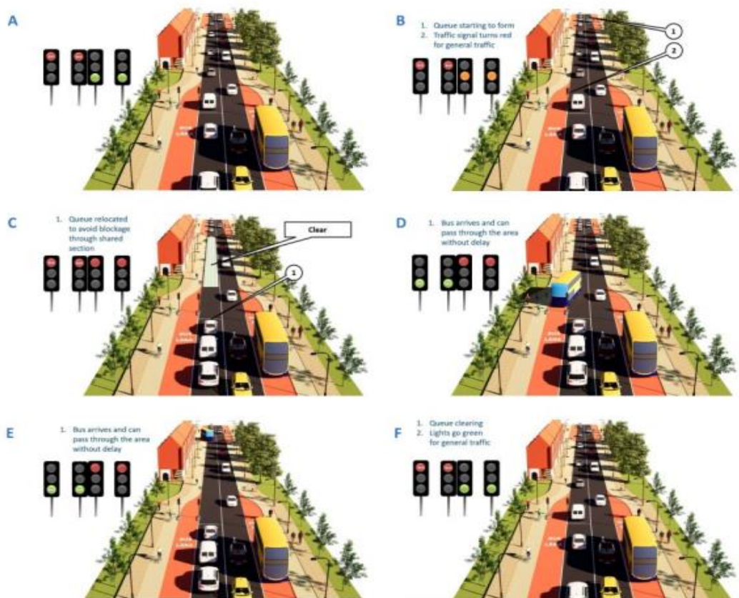
Image 4.18: Signal Controlled Priority Schematic Operation (Source: PDGB)
